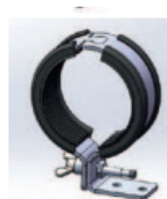
fixing clamp Ø70 mm, galvanised, angle plug, wall clearance 70 mm, mit distance bush
