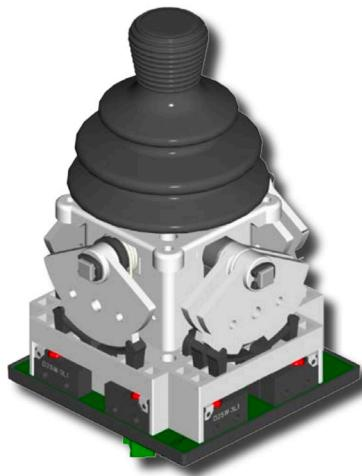
Juliet joysticks are control devices for all industrial machinery. They operate as auxiliary controllers of electrical motors through a power interface, such as a contactor. Designed for heavy duty use by qualified operators, Juliet is aimed specifically for the industrial market. Size and shape, resulting from a thorough analysis of the ergonomic features of the product, combined with the research of a graphic style suitable for a modern industrial environment, make Juliet easy to operate.
